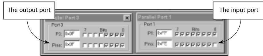
FIGURE 4.9 Running the code from Listing 4.5 in the simulator. Changing the status of the switch pin (Pin 1.0) alters the output on Port 3
