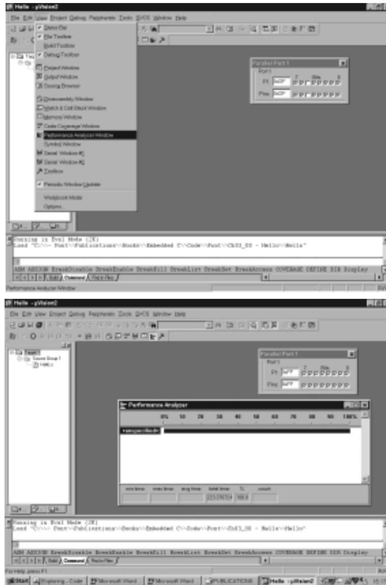
FIGURE 3.9 Running the Performance Analyzer in order to measure the duration of the loop delay function
