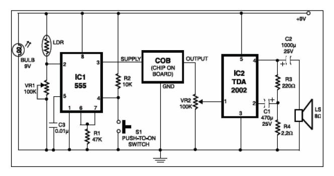
Everyone is aware that when anything catches fire, smoke is produced. When this smoke passes between a bulb and an LDR, the amount of light falling on the LDR decreases. This causes the resistance of LDR to increase and the voltage at pin 2 of IC 555 goes below 1/3 Vcc. thus triggering IC 555 which is used here in bistable mode. As a result the voltage of pin 3 goes high. This high voltage (approximately +9V) completes the supply to the COB (chip-on-board).
