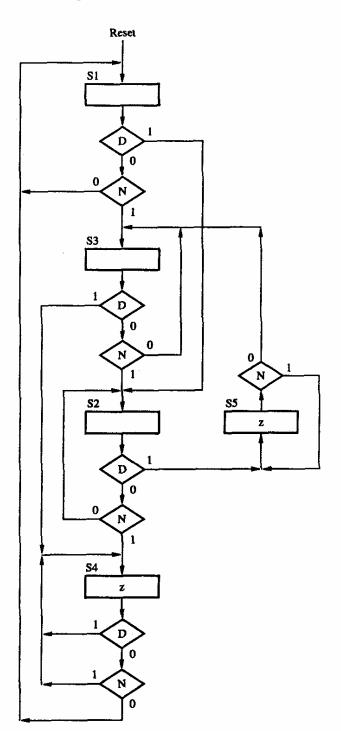
8.37. An ASM chart for the FSM in Figure 8.58 is
