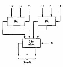
5.23. Using the approach explained in the solutions to problems 5.21 and 5.22, the desired circuit can be built as follows:
