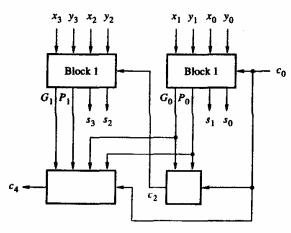
Blocks 0 and 1 have the structure similar to the circuit in Figure 5.16. The overall circuit is given by the expressions
