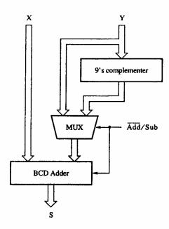
For the 9's complementer one can use the circuit designed in problem 5.18. The BCD adder is a circuit based on the approach illustrated in Figure 5.40.
