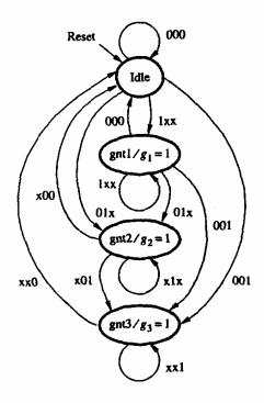
8.40. The required control signals can be generated using the following FSM:
