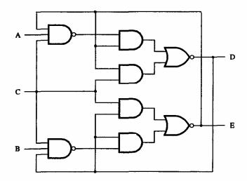
This modified circuit acts as a negative-edge-triggered JK flip-flop, in which J = A, K = B, Clock = C, Q = D, and  $\overline{Q} = E$ . This circuit is found in the standard chip called 74LS107A (plus a Clear input, which is not shown).
