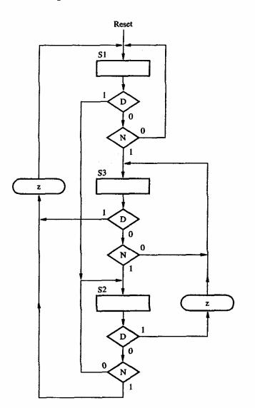
8.38. To ensure that the device 3 will get serviced the FSM in Figure 8.72 can be modified as follows:
