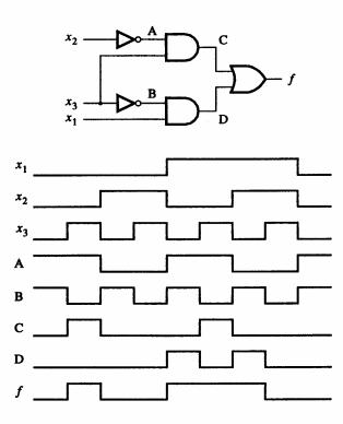
2.8. Timing diagram of the waveforms that can be observed on all wires of the circuit:
