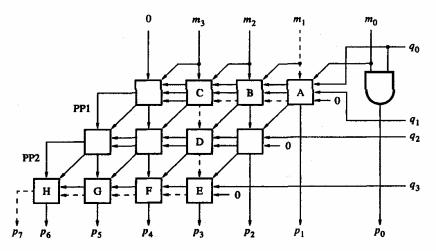
Propagation through the block A involves one gate delay in the AND gate shown in Figure 5.33b and two gate delays to generate the carry-out in the full-adder. Then, in each of the blocks B, C, D, E, F, G, and H, two more gate delays are needed to generate the carry-out signals in the circuits depicted by Figure 5.33c. Therefore, the total delay along the critical path is 17 gate delays.
