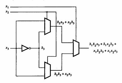
(b) Assuming the multiplexers are implemented using transmission gates
