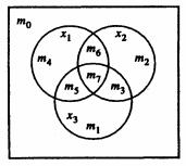
(b) For  $f = x_1 \overline{x}_2 x_3 + x_1 x_2 + \overline{x}_1 x_3$  have:
