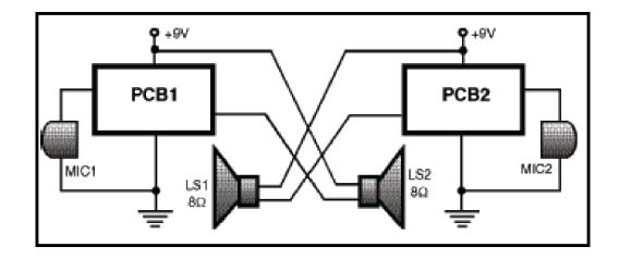
For making a two-way intercom, two identical units, as shown in figure, are required to be used. Output of one amplifier unit goes to speaker of the other unit, and vice versa. For single-battery operation, join corresponding supply and ground terminals of both the units together.
