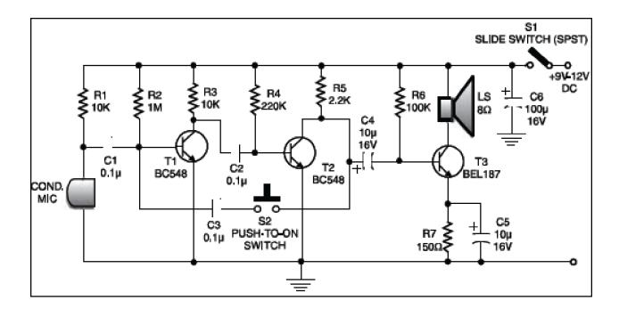
The circuit comprises a 3-stage resistor- capacitor coupled amplifier. When ring button S2 is pressed, the amplifier circuit formed around transistors T1 and T2 gets converted into an asymmetrical astable multivibrator generating ring signals. These ring signals are amplified by transistor T3 to drive the speaker of earpiece.
